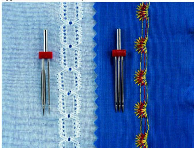
Fig. 11: left: DOUBLE HEMSTITCH NEEDLE, right: TRIPLE NEEDLE
